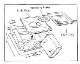
(1) Remove Chip Tray, Punching Plate and Sink Filter from oil tank.
