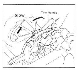
① Cut the thread exceeding Dies-wide while lifting up Cam Lever gradually.
